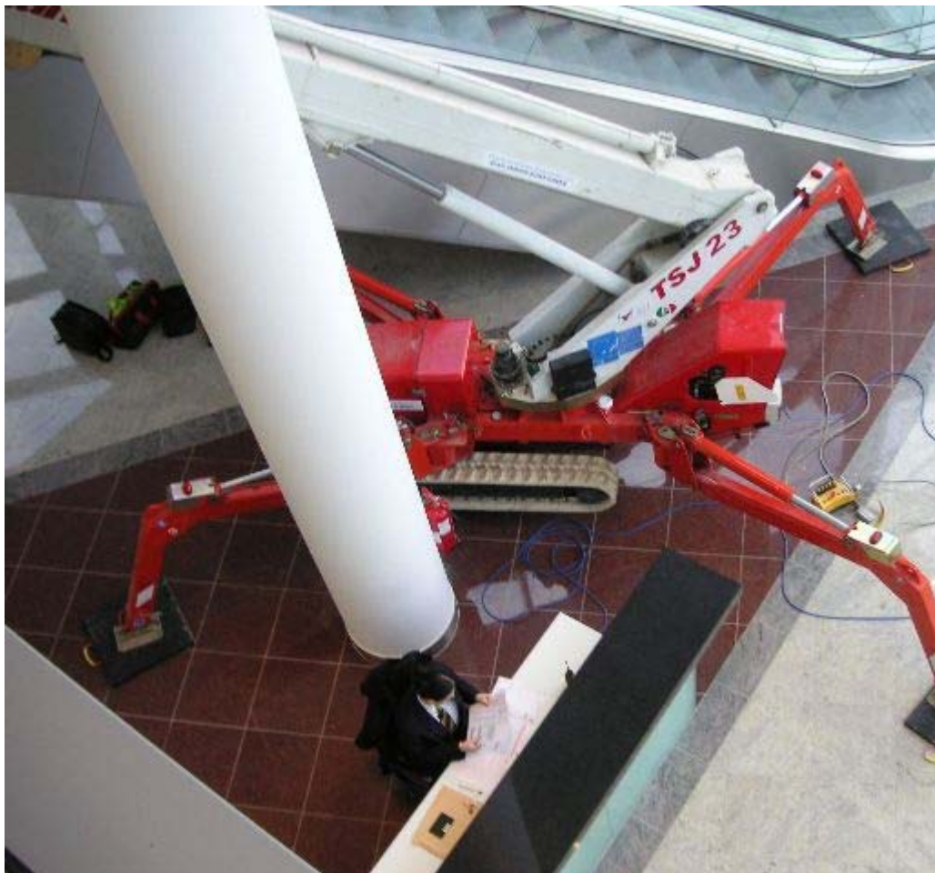
A Palazzani TSJ23 demonstrates the benefits of Spider leg outriggers
