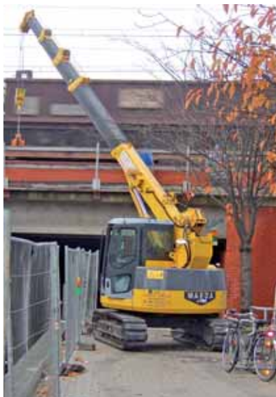
Midi tracked cranes – based on excavator bases – such as this Maeda LC-785 are larger but offer pick-and-carry duties.
